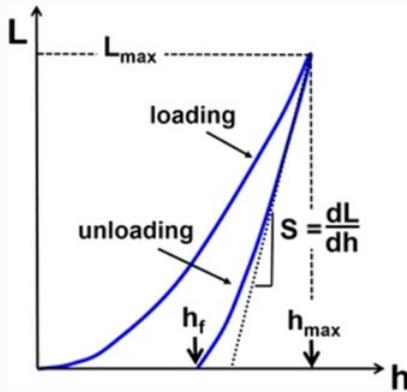
Figure 1: Load-unload curve during nanoindentation (Adapted from [8]).
