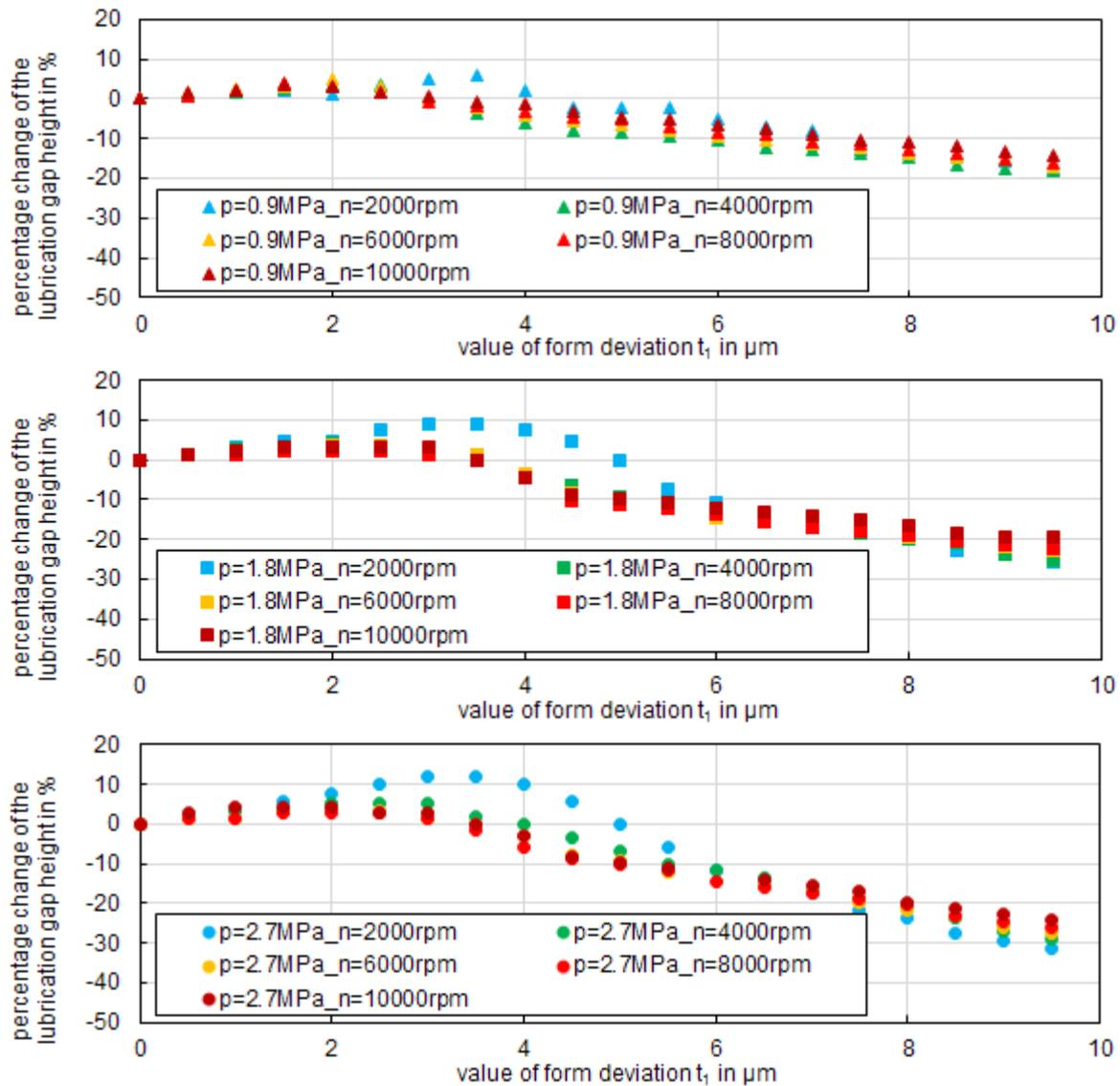
Figure 4: Minimum lubrication gap height of a three-sided-lobe bush at different form deviations in a best-case orientation scenario for a journal bearing with diameter  $d = 30$  mm, wide-to-diameter ratio  $b/d = 0.5$  and a relative bearing clearance of  $\psi = 2\%$
