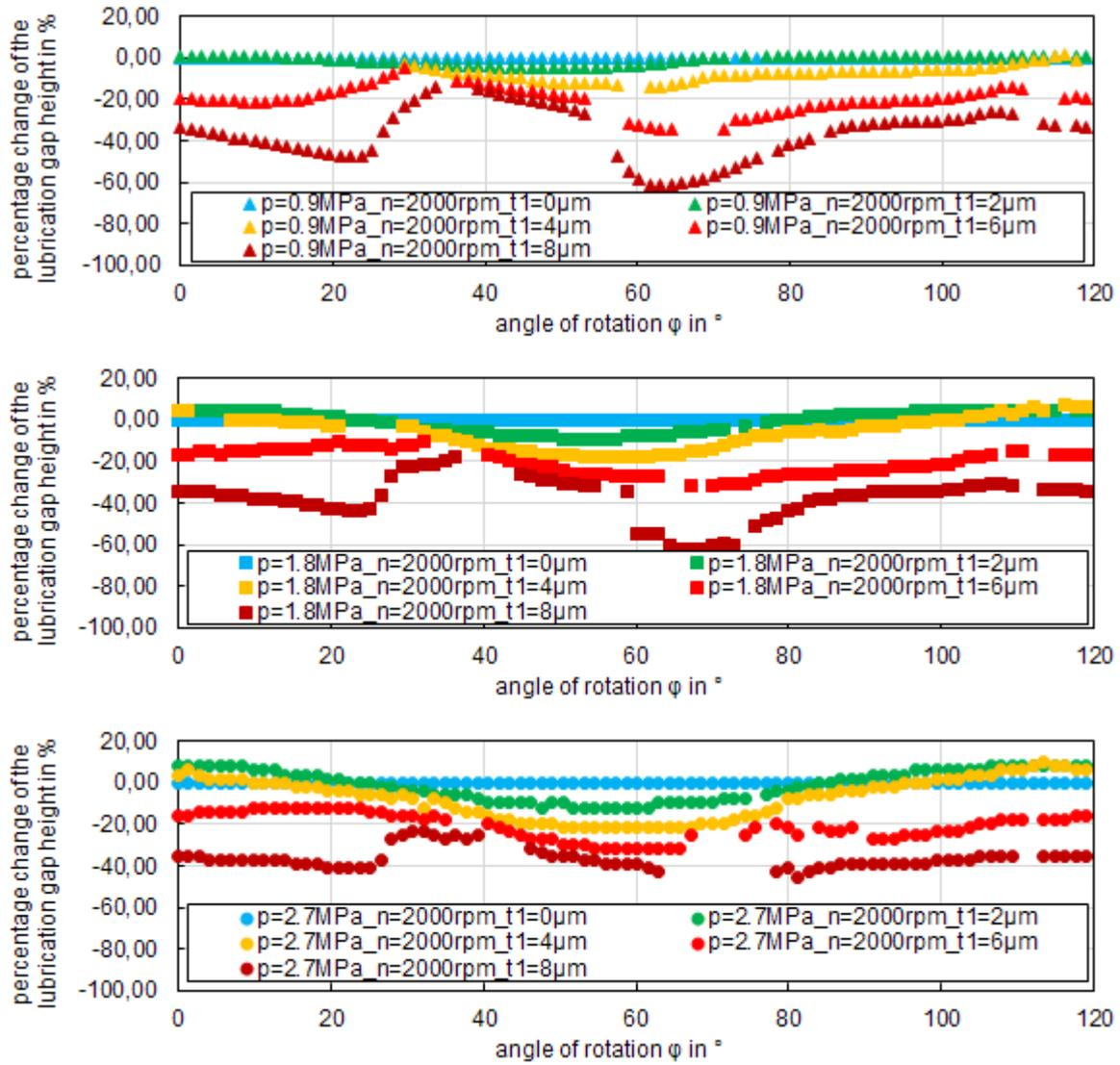
Figure 5: Minimum lubrication gap height of a three-sided-lobe bush at different form deviation values  $t_1$  at different rotation angles  $\phi$  or a journal bearing with diameter  $d = 30$  mm, wide-to-diameter ratio  $b/d = 0.5$  and a relative bearing clearance of  $\psi = 2\%$
