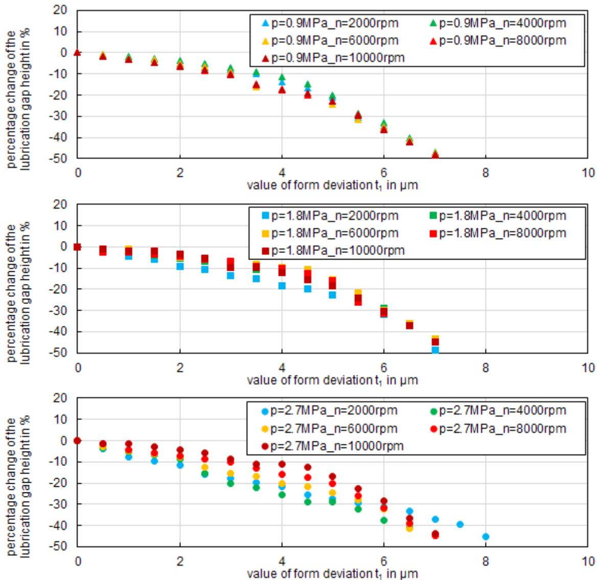
Figure 3: Minimum lubrication gap height of a three-sided-lobe bush at different form deviations in a worst-case orientation scenario for a journal bearing with diameter  $d=30$  mm, wide-to-diameter ratio  $b/d=0.5$  and a relative bearing clearance of  $\psi = 2\%$
