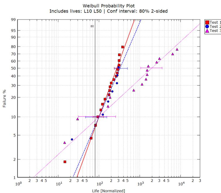
Figure 2 – Weibull plot for three tests (normalized)
