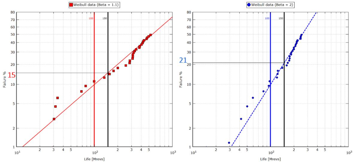
Figure 1-  $L_{10}$  estimation sensitivity to Beta (1.1 and 2)
